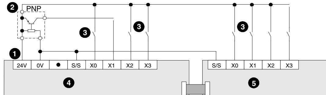
Figure 5.2: ENG Sink (negative input connection, positive S/S)
