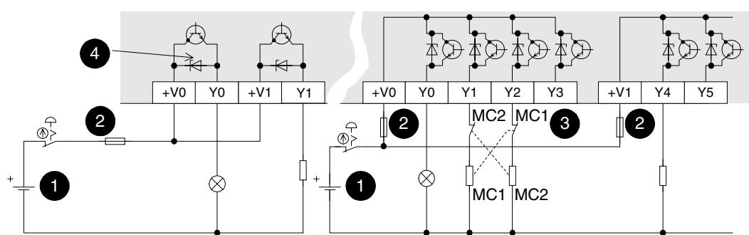
Figure 6.7: FX2N -☆☆MT, FX2N-☆☆ET (Sink) Japanese spec.
