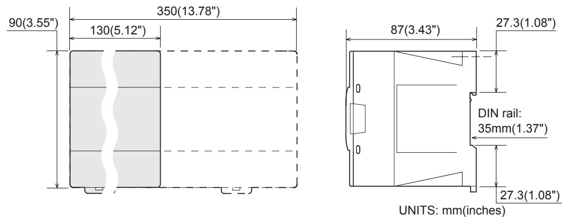
*Figure 1.2:* ENG Extension block dimensions
