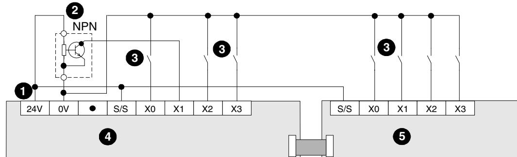
Figure 5.3: ENG Sink (negative input connection, Japanese spec.)
